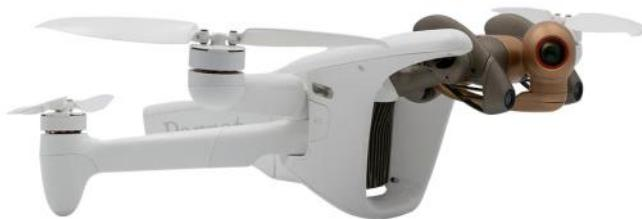
The Parrot ANAFI Ai is a 4G-connected drone designed for disaster planning and emergency management. Its robust connectivity ensures stable communication even in challenging environments. The 48 MP camera captures detailed imagery, aiding in damage assessment. Autonomous photogrammetry and obstacle avoidance enhance operational efficiency and safety. Its open-source platform allows for customized applications, making it a versatile tool for emergency response.
