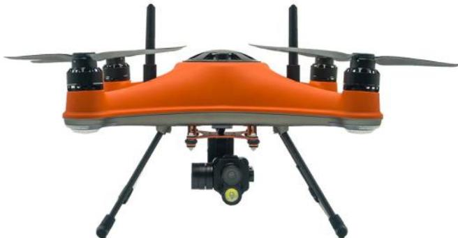
The Splash Drone 4 is designed for use near oceans and other water bodies. It boasts an IP67 waterproof rating, and its internal components are built to resist corrosion. This drone offers customizable options suitable for both leisure and emergency response purposes. Its payload release system can handle a 2-kilogram load, with a maximum flight duration of 30 minutes, enabling several drops within this time frame. Moreover, it can operate reliably in wind speeds of up to 38 mph.
