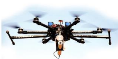
Cypher 6 with DroneRad Sensor
